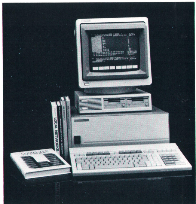
Fig. 1. The HP 4971S LAN Protocol Analyzer is designed for local area network troubleshooting and management. It can monitor and simulate network traffic and gather data independently of network hardware and software.
